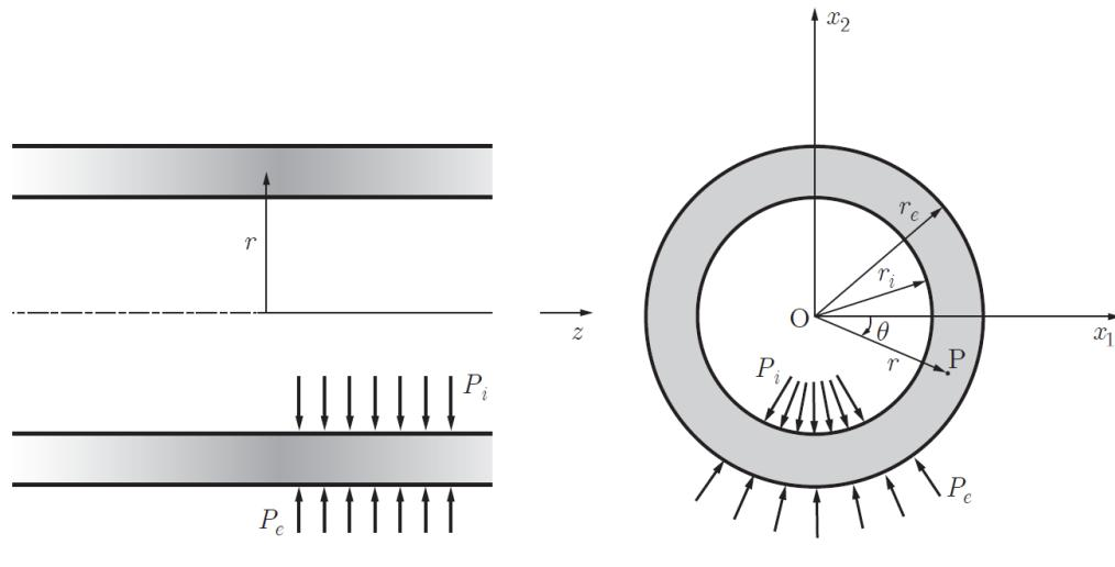
$$\sigma_{rr} = \frac{1}{r_e^2 - r_i^2} \left( r_i^2 P_i - r_e^2 P_e + \frac{r_i^2 r_e^2}{r^2} (P_e - P_i) \right)$$
